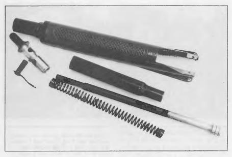
ABOVE: Type 63 gas system, showing gas regulator, regulator retaining pin, piston spring, piston, gas cylinder and upper handguard.
